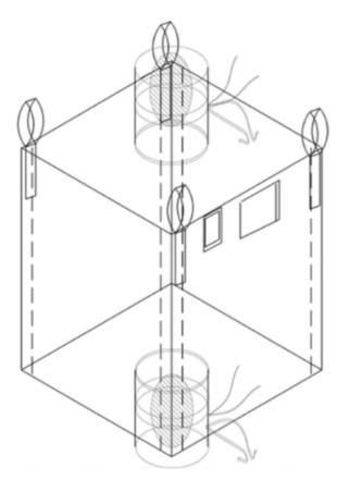
They are made with four individual pieces inserted to form a square structure. When filled, a 4-panel bag maintains its square shape similar to other types of construction. Typically, 4-panel bags hold their shape better than U-panel bags.
