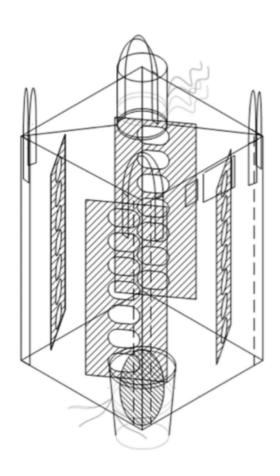
They are designed with filling and various unloading systems of types, each one special for the material it contains, and have lugs on the upper part to allow their transport.
